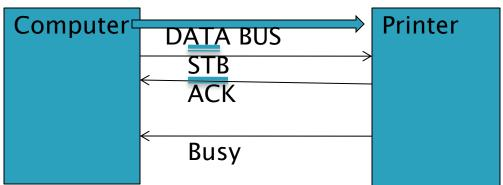
Handshaking signals is used to transfer data between whose data transfer is not same.
